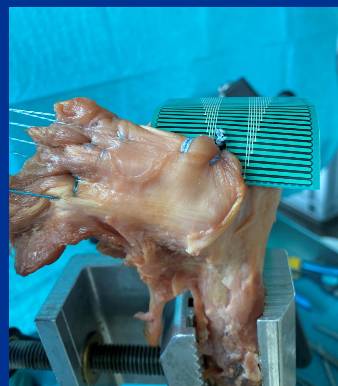
Fig. 3: Left cadaveric shoulder after knotless tape repair (group 3), illustrating the pressure-sensitive film placed between tendon and footprint.
