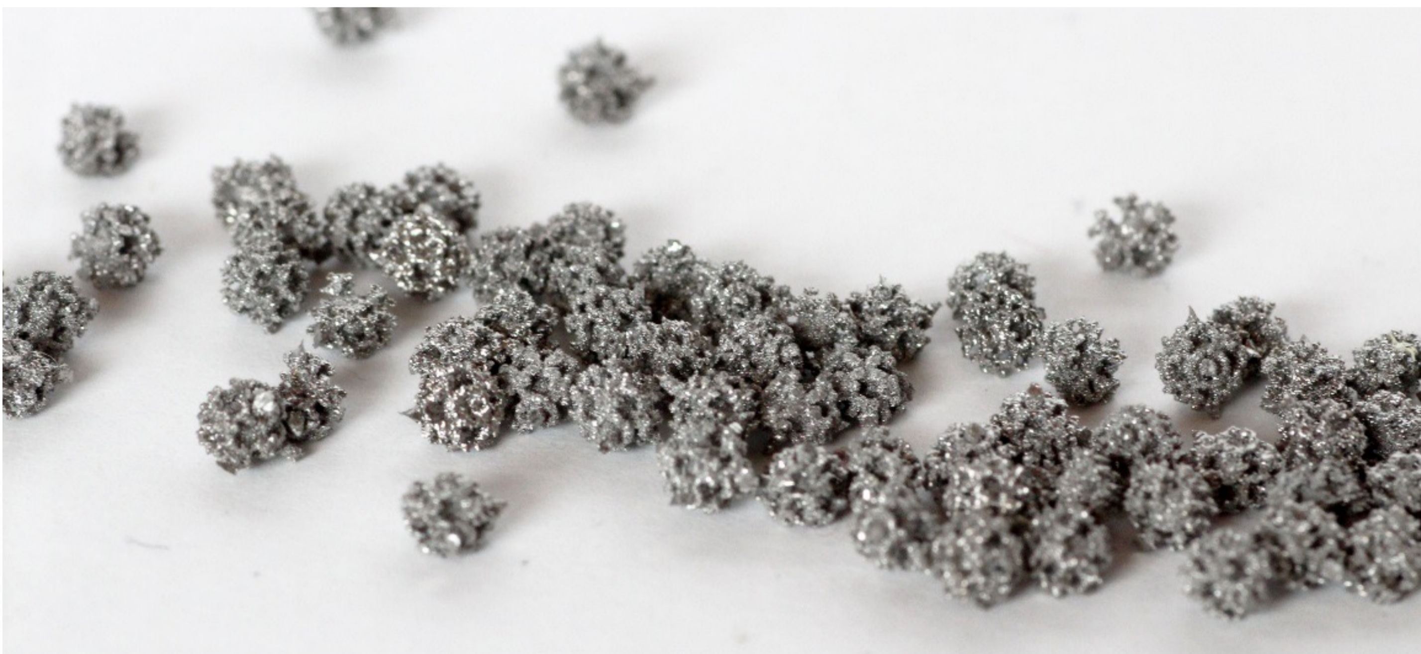
Titanium microspheres made by EBM® (Patent MT Ortho design)
